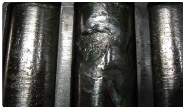
Damaged outer taper roller bearing
